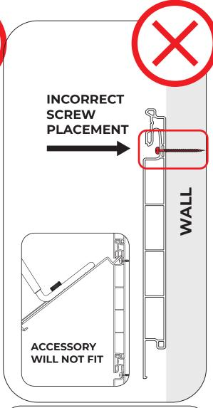
FRONT OF PANEL SHOULD BE FACING OUT WHEN INSTALLED
