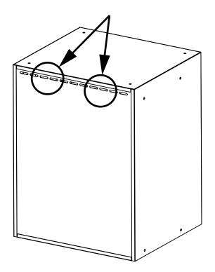
After securing the screws at the top,Mark and drill holes through the cabinet. These holes should be lined up with the top screws to completely secure the cabinet to the wall.
